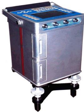
Figure 12. View of the Canadian-made CG-5 AutoGrav type gravimeter under research.
